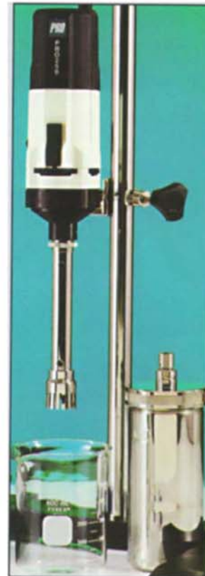
CHEF BOYARDEE in-can homogenizes ravioli, tortellini and other pastas for compositional analysis using a customized PRO 250 lab homogenizer
