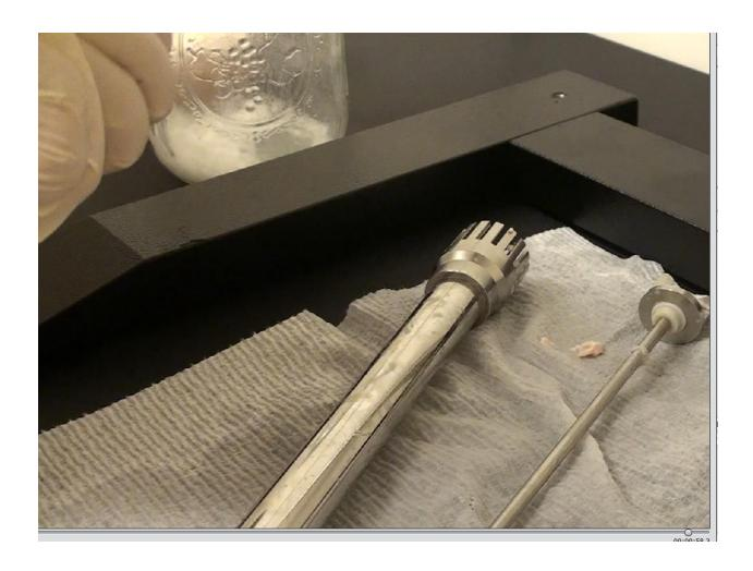
The generator is shown disassembled with the only remaining fibrous components left. Notice the significant decrease in size compared to large batch processing with a generator probe only.
